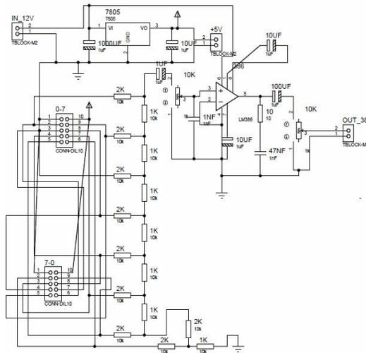
Figure 4 Schematic of the modulator
