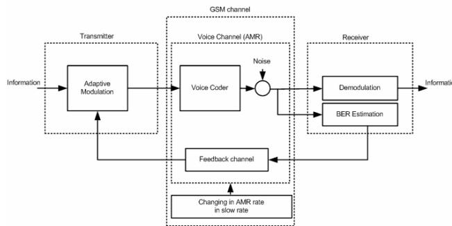
Figure 2 Proposed adaptive modulation with feedback channel
