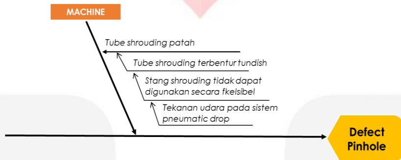
Gambar 6 Diagram Fishbone Defect Pinhole
