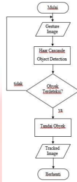
Gambar 6 Diagram Alir Hand Detection Haar Cascade
