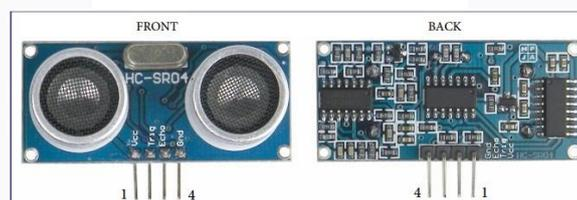
Gambar 2 Sensor Ultrasonik
