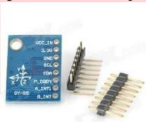
Gambar 2. Sensor IMU MPU6050
