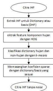
Gambar 3.3 Blok diagram proses penghilang *noise*
