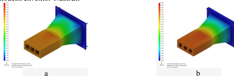
Gambar 19 Total Deformation Molding Briket Eksisting (a), Total Deformation Molding Briket Usulan (b)
