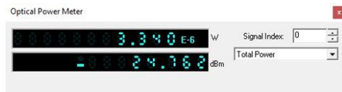
Gambar 4. 2 Hasil Power Received Terburuk Pada Link Backhaul
