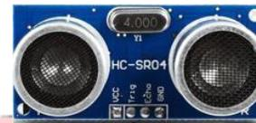
Figure 5 Ultrasonic Sensor
