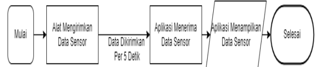
Gambar 3. 7 Flowchart penerimaan data sensor
