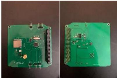
GAMBAR 5. PCB MODUL KOMUNIKASI RFM69HW
